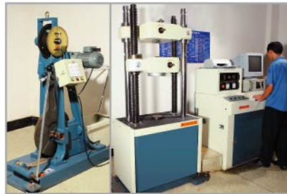
Charpy Impact Testing Machine 沖擊試驗機 Universal Testing Machine (Tensile, Yield Strength...etc) 拉伸試驗機
